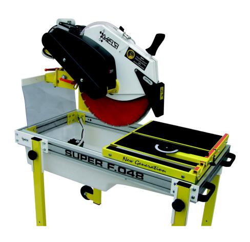
Ideal for cutting bricks, stones, Poroton and other building materials — up to 19 cm in a single pass.
