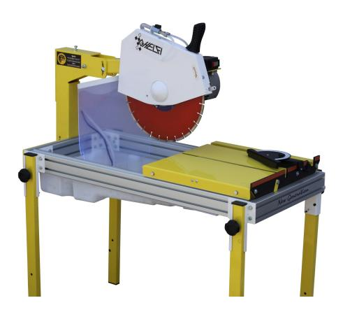
Ideal for cutting bricks and other building materials — up to 14 cm in a single pass.
